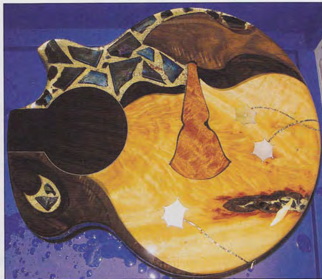
Above: Final resin coat on body blank for Tiffany Prototype, with glass and inlays. Below: Final coat on blank for N11, Loetz Gilded Serpent.
