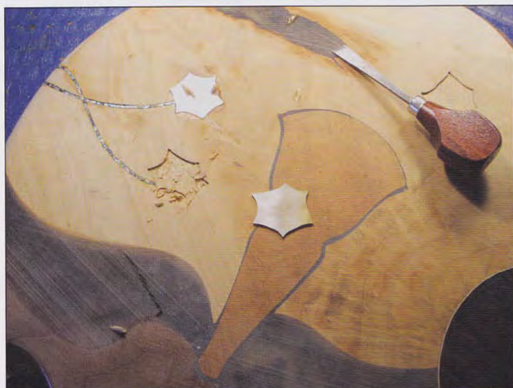
Installing flower inlays on the sanded blank for Tiffany Prototype.
