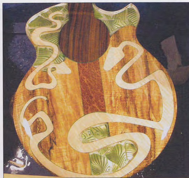
Above: Final resin coat on body blank for Tiffany Prototype, with glass and inlays. Below: Final coat on blank for N11, Loetz Gilded Serpent.
