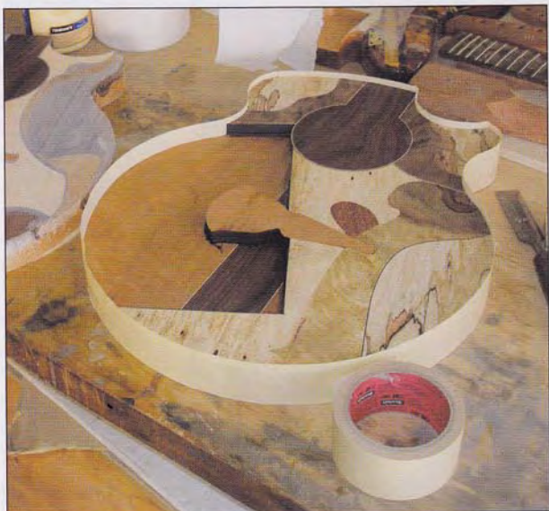
Prepping body for N4, Lautrec Yvette for the first coat of resin. N4 will feature a print by Henri de Toulouse-Lautrec.
