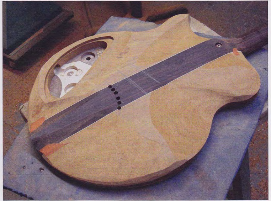
Shaping a back. The contours expose the stringers that key the mahogany to the rosewood.
