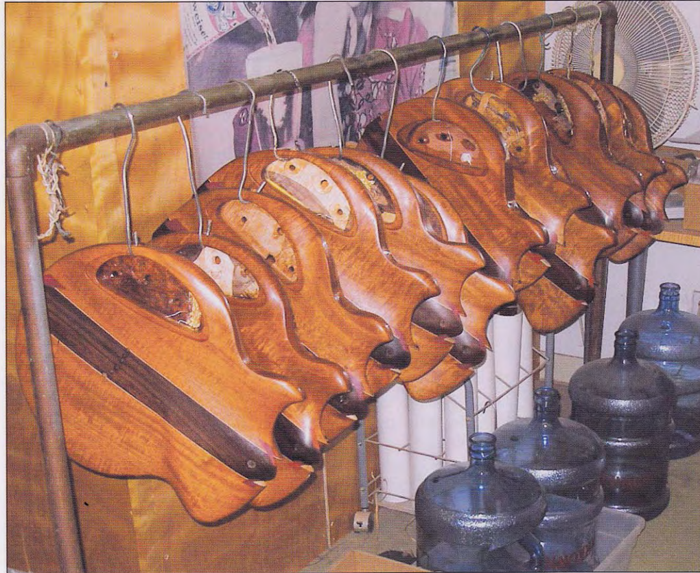
Top, left: Marking for saddle pieces. Top, right: Finished bridge. Above: While the tops of the Nouveau guitars were coated with resin, the backs were finished with Formby's tung oil after being shaped and sanded. A mixture of two parts gloss oil and three parts semigloss was used.
