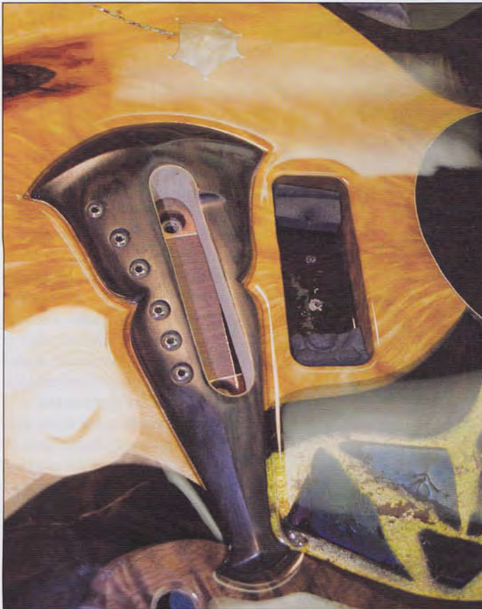
Bridge surround set into wet resin on Tiffany Prototype.
