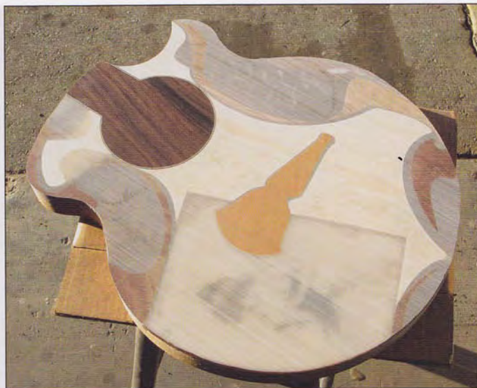
Resin covered sanded body blank for N1.
