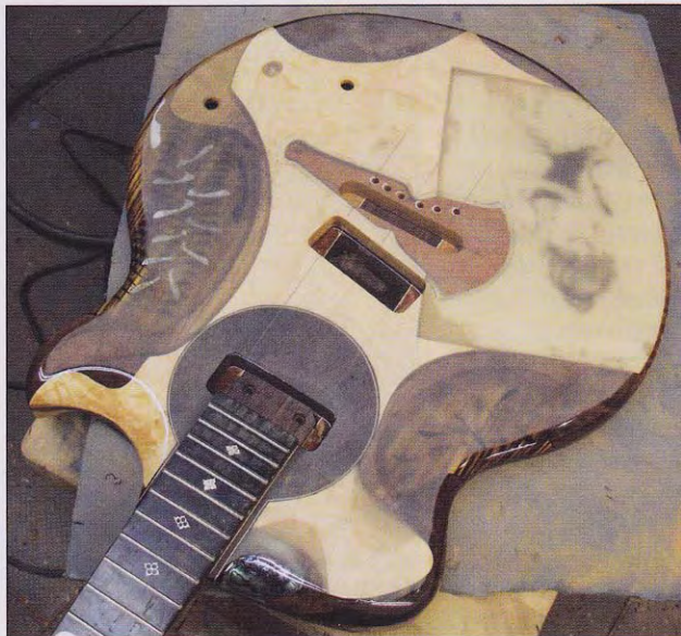
Middle, left: The neck pocket is laid out. The resin can be marked with a scribe. The scratches will disappear with the next coat. Center: The neck pocket is cut. Middle, right: Inserts for the two inside neck bolts. Bottom, left: Spider inlay in neck for N10, Spinning Arachnid. Bottom, center: The pickup cavities and bridge placement are scribed and routed in N1. Note the bolt holes in the upper end of the neck. Bottom, right: Contoured body with neck attached showing the single visible neck bolt in the three-bolt system.
