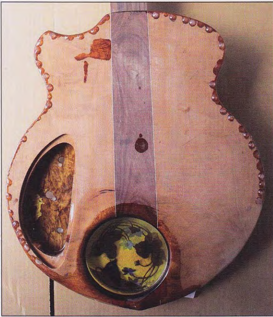
View of a back. The resin drips around the edge are visible.
